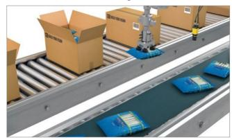
In-Sight 2D vision systems locate and identify objects for pick-and-place robotic packing.
