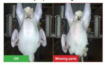
Al-based vision systems identify missing legs or wings, inspect for tearing, bruising, and color.
