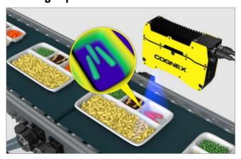
3D displacement technology inspect portion sizes prior to packaging.
