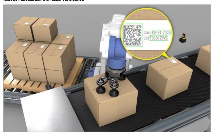
In-Sight 2D vision systems verify 2D and alphanumeric codes on cartons and guide robotic arm for palletizer.
