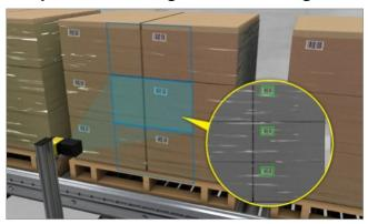
DataMan barcode readers combined with High-Speed Steerable Mirror simultaneously read multiple codes on pallets.
