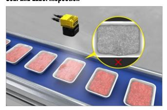
Al-based vision systems check the integrity of film seals on trays and read product labels and codes to prevent mislabeling.
