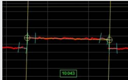
Measures the width of a strip.
